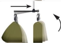
If the spindle is moved forwards, the arm and the hand can be tilted upwards more easily.
