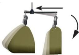
The more the spindle is moved backwards (i.e. towards the elbow), the easier the arm and hand can be tilted downwards.
